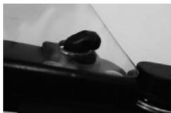
2. Guide the visor around the holder, placing the holes over the positioning pins.
