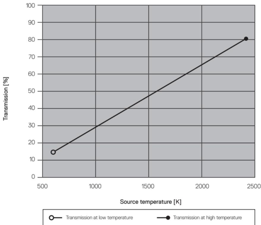
As you can see from the graph, the protection HighTemp visors provide against radiant heat depends on how hot the heat source is. The higher the temperature, the higher the damaging heat that hits the eyes. The visor should only be used in situations where it can limit the exposure of the wearer's eyes to less than  $100 \text{ W/m}^2$ .
